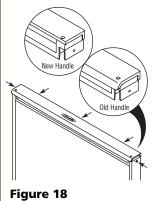
4. Remove the three screws located on the back of the handle (see **Figure 18**).
